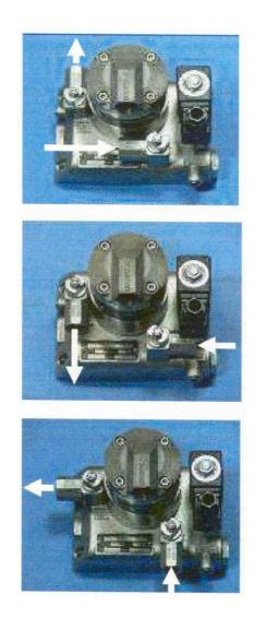
Shown above, each of the inlet & outlet valve assemblies may be repositioned in one of three 90 degree incremental positions by accessing the socket head screws on the underside of the manifold.
