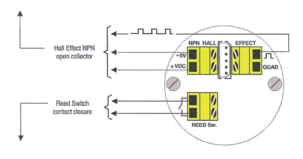
**2.3.2** Reed Switch Pulse Output The reed switch output is a two wire normally open SPST voltage free contact ideal for installations without external power or for use in hazardous area locations when Intrinsically Safe (I.S.) philosophy is adopted. Note: when using the reed switch output the liquid temperature must not change at a rate greater than 10°C per minute (50°F per minute). In general the reed switch life will exceed 2 billion actuations when switching less than 5Vdc @10mA.
