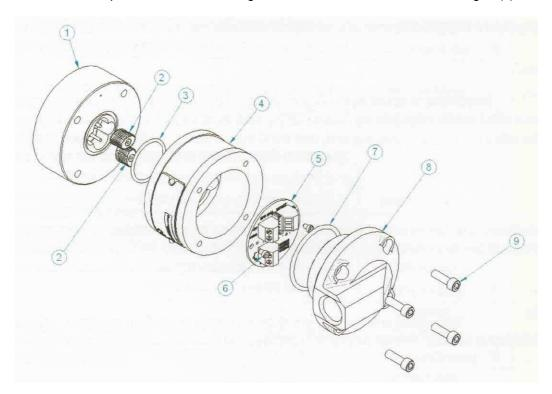
**4.5 Inspection** Remove, inspect and clean the rotors, also check that the magnets have not been chemically attacked. Check the measuring chamber for damage or scoring & redress if necessary, the rotor shafts should NOT be loose or able to be rotated.
