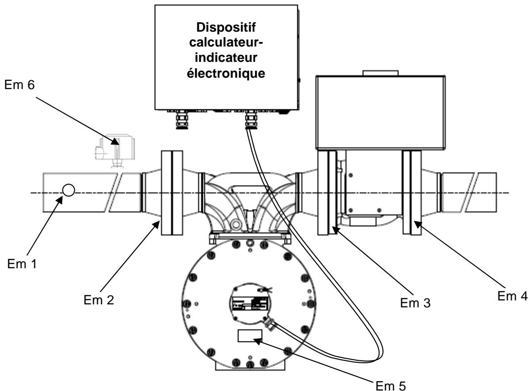
The meter, the automatic gas detection and evacuation display and the stopping automatic valve can be mounted in horizontal or vertical position.
