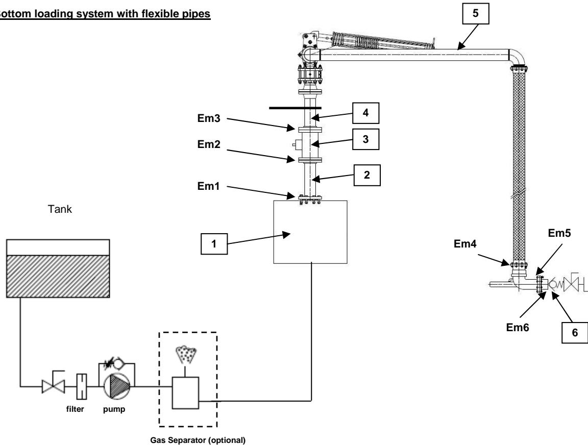
Sealing plan of SATAM measuring system
