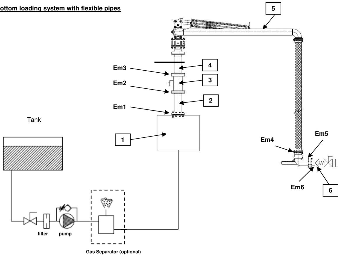
Sealing plan of SATAM measuring system
